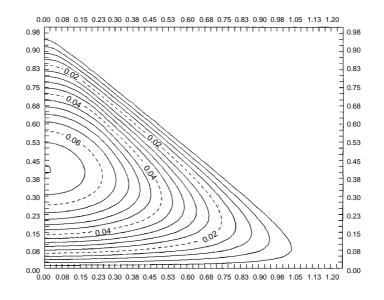
**Figure 3.** Velocity field inside an isosceles triangular duct (1/m = 1.25)
