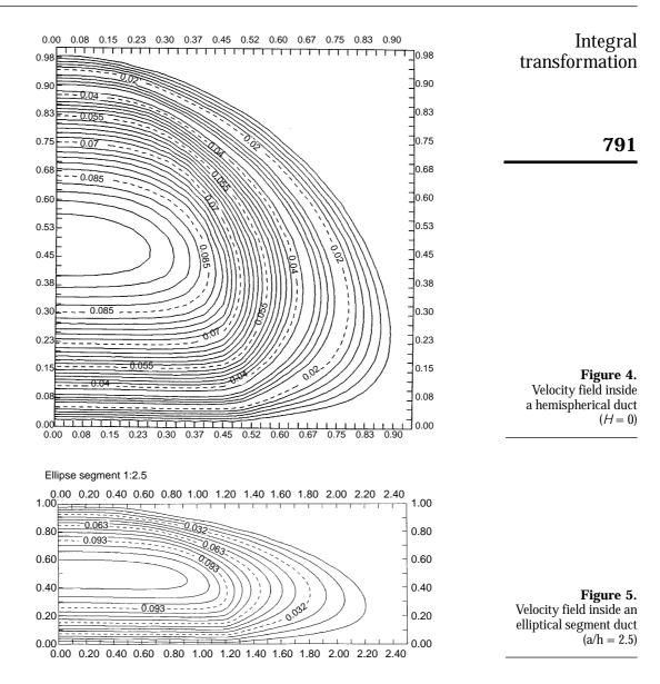
some representative values of the governing geometric parameters, namely, 1/m = 1.25 for the isosceles triangular duct, the hemispherical segment duct, and a/h = 2.5 for the elliptical segment duct, which serve to demonstrate the absence of oscillations in the eigenfunction expansions representations of the potential, over the entire solution domain.
